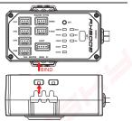
Turn on the GOOSKY T8 transmitter, press the BIND button for 3 times after the helicopter is powered on. The blue light flashes quickly. Keep the transmitter less than one meter away from the flight control. The flight control passes self-detection when the blue light is solid on. Then the binding is done.
