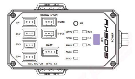
Bind the transmitter to the aircraft (wait for the flight controller initialization to complete), and then press the SET button 10 times. At this time, the flight controller indicator LEDs flash red and blue together. After the flight controller initialization is completed, the factory settings are restored.
